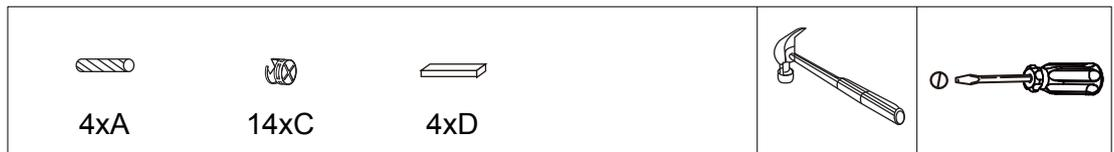
STEP 2: Attach panel (1)&(2) to the body, using dowel (A) and cam lock (C). Attach non-slip sticker (D) to panel (1)&(2).
